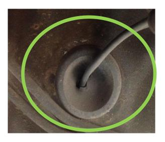
If your vehicle does not have any suitable pre-existing methods to route your BMC01 cable into the cabin of the vehicle, make sure when you run the wiring that it's via rubber grommet(s) to protect the vehicle and the new wiring.
